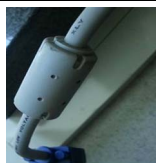
Figure 10 VGA cable with thicker EMI core
