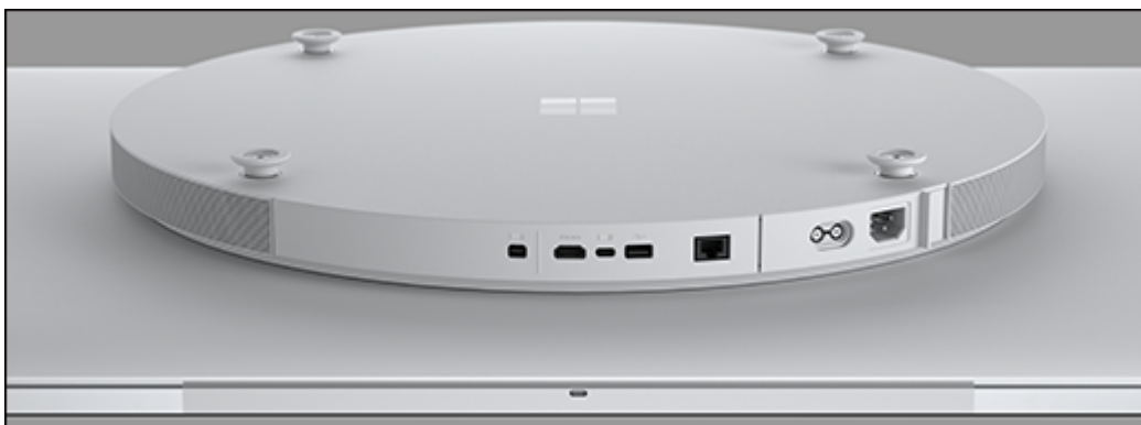
Figure 3. View of compute cartridge on the bottom of 50" models of Surface Hub 2S or Surface Hub 3.
